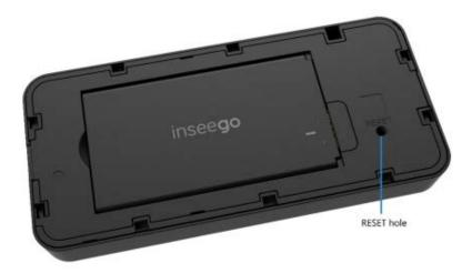
Place one end of an unfolded paper clip into the RESET button hole and press until the screen displays M2000 Resetting (about five to six seconds). Your M2000 restarts with factory settings.
